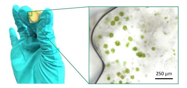
The image shows a section taken of the photosynthetic engineered living material. On the right side of the picture clusters of algae cells are shown which convert sunlight,  $CO_2$  and water into glucose. Credit: Delft University of Technology
