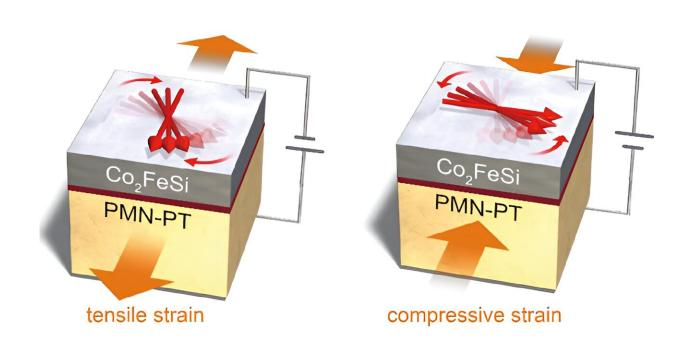
Interfacial multiferroic structure and control of magnetization orientation. Credit: *NPG Asia Materials* (2024). DOI: 10.1038/s41427-023-00524-6
