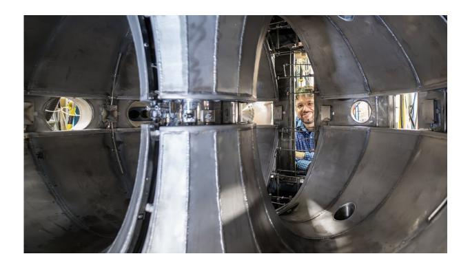
This view of the inside of LTX-β shows what the donut-shaped plasma containment device looks like after the lithium has been cleaned off the shell walls and several ports were opened. PPPL Staff Research Physicist Dennis Boyle peeks in from center-right. Credit: Elle Starkman/PPPL Office of Communications
