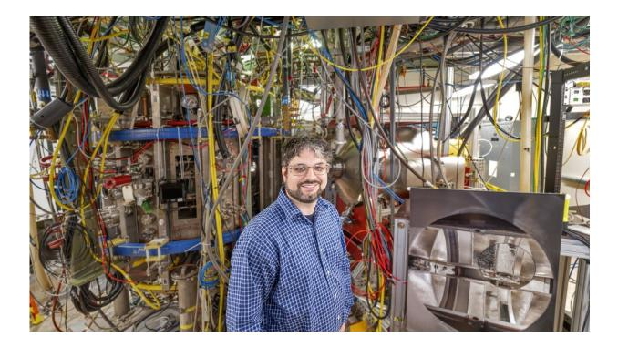
Dennis Boyle, a staff research physicist at PPPL, stands in front of LTX- $\beta$ . The plasma containment device requires a complex web of cables and hoses to operate. The beam system is to the right of Boyle's head. In the foreground on the right sits a photograph of the inside of LTX- $\beta$ , with an image inset showing a small pool of lithium. Credit: Elle Starkman/PPPL Office of Communications
