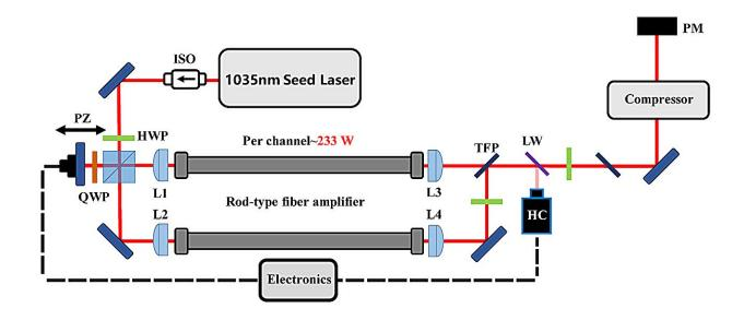
Diagram of coherent beam combining experimental setup. Credit: Shuangxi Peng, Zhihao Wang, Feilong Hu, Zhengyan Li, Qingbin Zhang, Peixiang Lu
