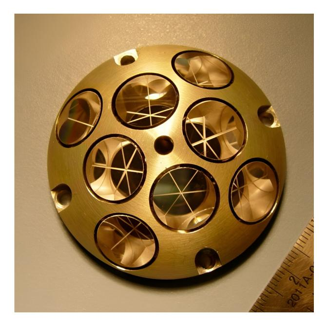
Only 2 inches, or 5 centimeters, wide, NASA's Laser Retroreflector Array has eight quartz-corner-cube prisms set into a dome-shaped aluminum frame. This configuration allows the device to reflect light coming in from any direction back to its source. Credit: NASA's Goddard Space Flight Center
