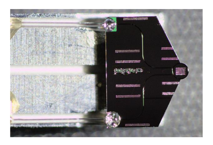
Photonic chip used in this study, mounted on a transmission electron microscope sample holder and packaged with optical fibers. Credit: Yang et al. DOI: 10.1126/science.adk2489
