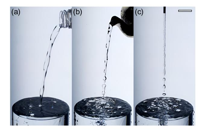
Water pouring on a filled cylindrical cup from (a) a commercial plastic bottle and (b) a teapot. (c) Model water pouring from a smooth brass tube. Scale bar: 2 cm. Credit: *Physical Review Fluids* (2023). DOI: 10.1103/PhysRevFluids.8.L122002
