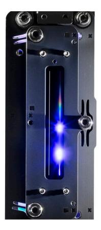
Researchers at Fraunhofer IOF have developed and manufactured a highprecision silicon-based double slit for the spectrometer on board ESA's FLEX satellite Credit: Fraunhofer IOF
