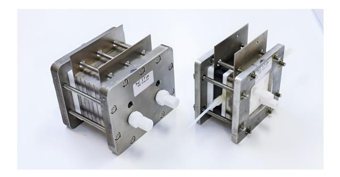
Comprising a sandwich-structured membrane electrode-assembly with a combined anion- and proton exchange membrane separating the cathode and anode, it converts  $CO_2$  into ethylene. Credit: Hong Kong Polytechnic University
