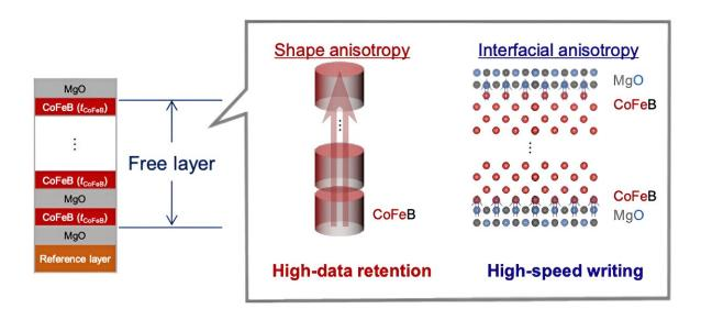
A film stack of the developed MTJ with the multilayered ferromagnetic structure. Shape anisotropy is enhanced by increasing the thickness of CoFeB and decreasing the number of CoFeB/MgO layers. Interfacial anisotropy is enhanced by increasing the number of CoFeB/MgO layers. Credit: Junta Igarashi, Butsurin Jinnai, and Shunsuke Fukami. From *npj Spintronics* (2024). DOI: 10.1038/s44306-023-00003-2
