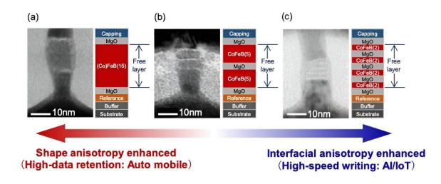
Cross-sectional transmission electron microscope images of the fabricated MTJs and their film stacks. Varying the number of CoFeB/MgO layers and the CoFeB thickness can tailor MTJ performance for retention-critical to speed-critical applications. Credit: Junta Igarashi, Butsurin Jinnai, and Shunsuke Fukami. From *npj Spintronics* (2024). DOI: 10.1038/s44306-023-00003-2
