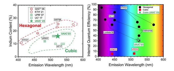
Closing the green gap: green emission with only 16% indium content which is much lower than hexagonal phase materials (left) and 32% IQE which is comparable to hexagonal phase materials and higher than conventional cubic active layers (right) Credit: University of Illinois Grainger College of Engineering
