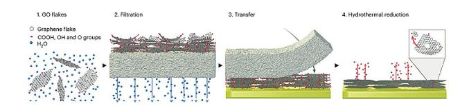
Preparation of the porous reduced GO thin-film EGNITE. This consists of filtering a GO solution through a porous membrane (1, 2), transferring the deposited film of stacked GO flakes onto a conductive substrate (3) and the hydrothermal reduction of the ensemble, which turns the film highly porous and conductive (4). Credit: *Nature Nanotechnology* (2024). DOI: 10.1038/s41565-023-01570-5
