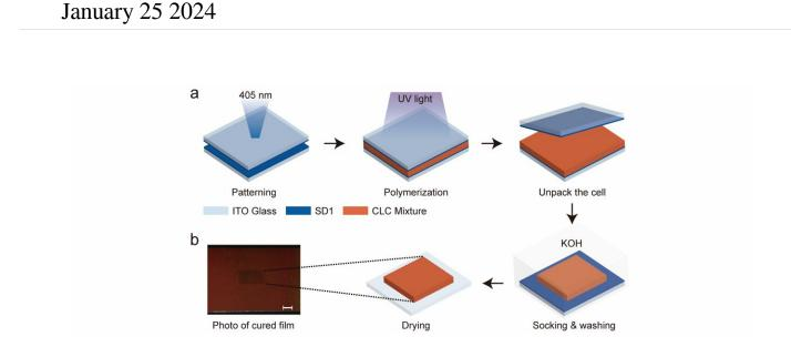
Fig. 1. a, fabrication process of humidity-responsive CLCP films with geometric phase encoding. b, Photo of the films cured at 65°C. The scale bar is 1 mm. Credit: Shi-Long Li, Zhao-Yi Chen, Peng Chen, Wei Hu, Chaohong Huang, Sen-Sen Li, Xuejia Hu, Yan-Qing Lu and Lu-Jian Chen
