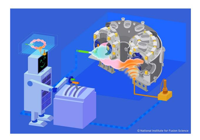
Image of digital twin control, in which real plasma is controlled by virtual plasma reproduced on a computer. In this research, we developed a digital twin control system that can estimate optimal control inputs while optimizing the virtual plasma by real-time observations and demonstrated its control capability through experiments at the LHD. Credit: National Institute for Fusion Science
