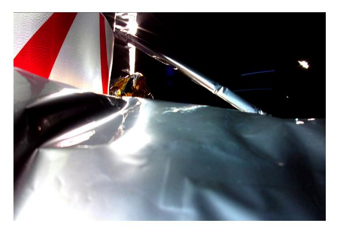
In this image released by Astrobotic Technology, an image from a mounted camera shows a disturbed section of insulation on the Peregrine lander, while on its way to land on the moon, Monday, Jan. 8, 2024. Credit: Astrobotic Technology via AP
