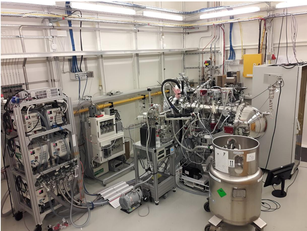
The photoelectron spectroscopy instrument was built at Stockholm University and allows studies of catalyst surfaces under high pressures. Credit: Peter Amman
