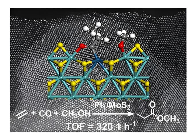
Pocket-like ensemble of Mo-S-Pt<sub>1</sub>-S-Mo sites for ethylene methoxycarbonylation by M-H mechanism. Credit: Wang An
