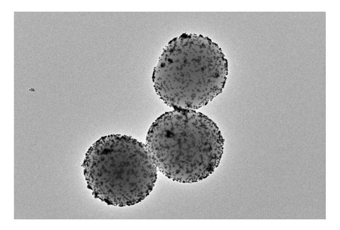
Transmission electron microscopy image of the nanorobots. Credit: Institute for Bioengineering of Catalonia (IBEC)
