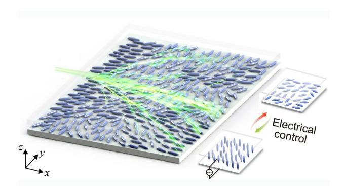
A schematic illustrating the branched flow of light in an NLC film. The random orientation of NLC molecules within a glass cell can be adjusted using an electrical voltage bias. Credit: Chang, Ss., Wu, KH., Liu, Sj. et al/*Nature Communications*. 10.1038/s41467-023-44500-8.
