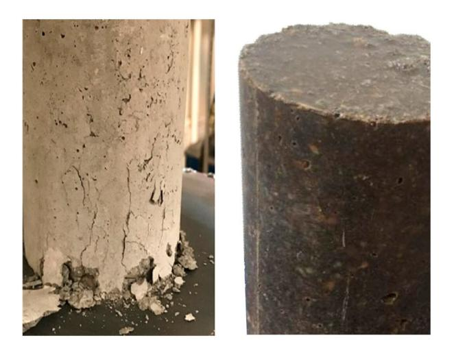
The provided laboratory samples, including conventional concrete with light color in the left side and polymer concrete with dark color in the right side. Credit: *Polymers* (2023). DOI: 10.3390/polym15193939
