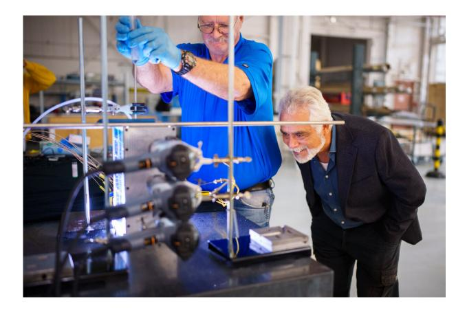
Sal Rodriguez, right, looks on in amazement as technologist Robin Sharpe injects dye into the dimpled model they built, showing the way dimples increase heat transfer in water. Credit: Craig Fritz/Sandia National Labs
