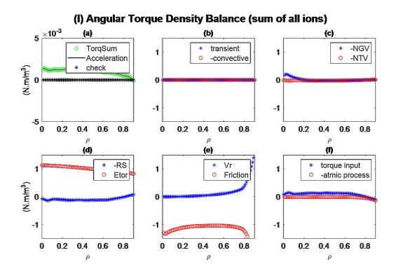
Relative comparison of all torque terms in fluid-based angular momentum balance of toroidally rotating tokamak plasmas. Credit: Bae Cheonho
