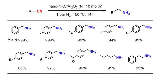
Hydrogenation of various nitriles using the nano-Ni<sub>3</sub>C/Al<sub>2</sub>O<sub>3</sub> catalyst under 1 bar  $H_2$ . Credit: 2024 Yamaguchi et al., Nickel Carbide Nanoparticle Catalyst for Selective Hydrogenation of Nitriles to Primary Amines, *Chemistry—A European Journal*
