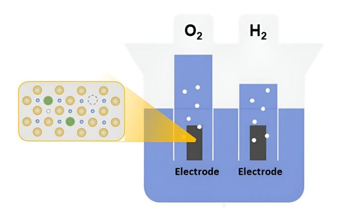
OER is important for the sustainable production of hydrogen via proton exchange member water electrolysis. Now, researchers present a novel  $RuO_2$ catalyst, stabilized by single atoms of zinc, for OER in proton exchange membrane water electrolysis. Credit: Haeseong Jang/Chung-Ang University
