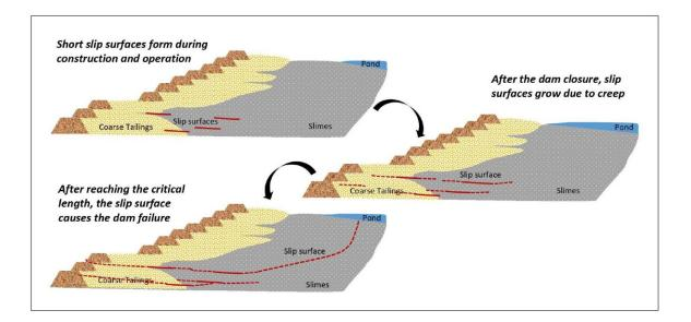
During construction, short slip surfaces formed in the deposits of the tailings dam (above). These grew after decommissioning due to creep deformation (centre) and reached the critical length (bottom) that caused the collapse of the dam. Credit: IGT/ETH Zurich
