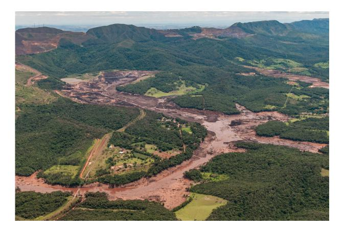
Image of the devastation two days after the dam collapse in January 2019. Top left: The leaking tailings pond. Bottom left: The destroyed railway bridge. Credit: Ibama from Brasil—Brumadinho, Minas Gerais, CC BY-SA 2.0, Wikimedia Commons
