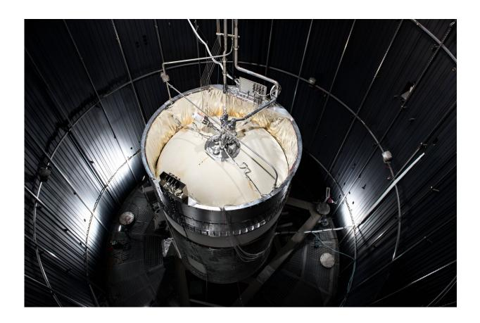
A 2019 image of the SHIIVER tank sitting inside the In-Space Propulsion Facility's vacuum chamber at NASA's Neil Armstrong Test Facility in Sandusky, Ohio. The tank was part of a Cryogenic Fluid Management project effort to test the tank at extreme temperatures and ensure the new technologies kept the propellants inside cold and in a liquid state. Credit: NASA
