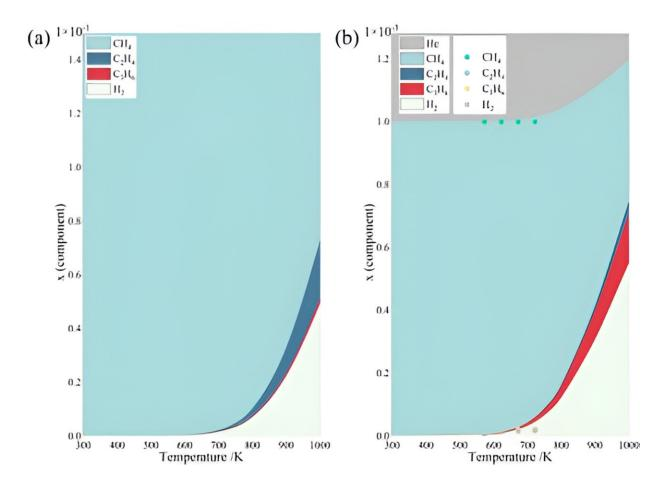
The equilibrium composition diagram for consecutive NOCM processes at (a) 1 atm with 100% methane initial; (b) 1 atm with 0.1% methane and 99.9% He initial. The deep colored points in (b) correspond to the experiment data. Credit: *Research*
