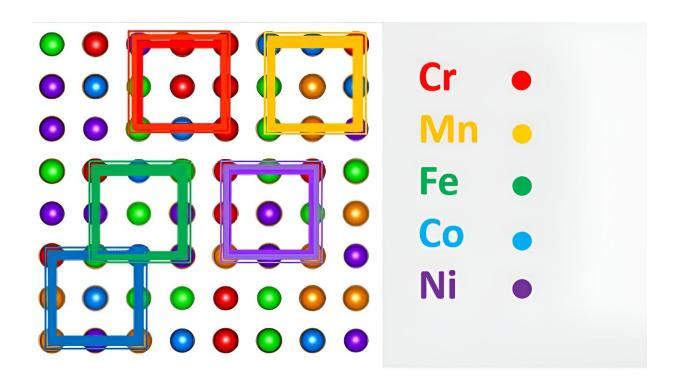
The analysis of the EXAFS data showed different local environments around the elements of the Cantor alloy depending on the annealing temperature, which indicate different ordering and diffusion processes. Manganese diffuses fastest in the high-temperature state, nickel in the low-temperature state. Credit: HZB
