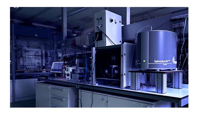
RoboChem is an autonomous benchtop platform for fast, accurate and aroundthe-clock chemical synthesis. Credit: University of Amsterdam
