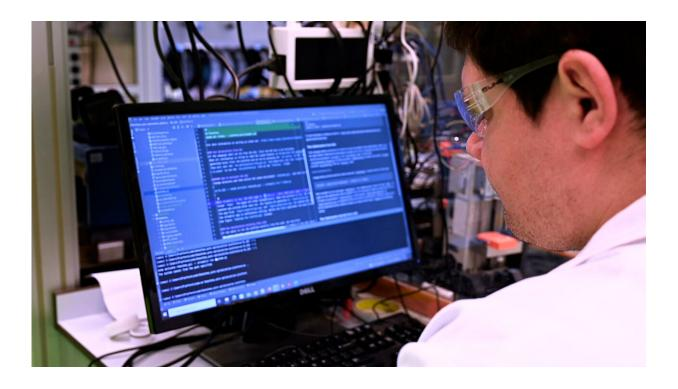
RoboChem applies a machine-learning algorithm that processes the data obtained from the system. It decides which reactions to execute, always aiming for the optimal outcome. Human intervention only takes place at the beginning, setting up the stock solutions and starting the RoboChem session. Credit: University of Amsterdam
