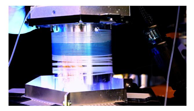
At the heart of RoboChem is a powerful photochemical reactor featuring an array of very powerful LEDs that illuminate the reaction solution. Here the molecules are transformed according to the instructions from the AI controller. Credit: University of Amsterdam
