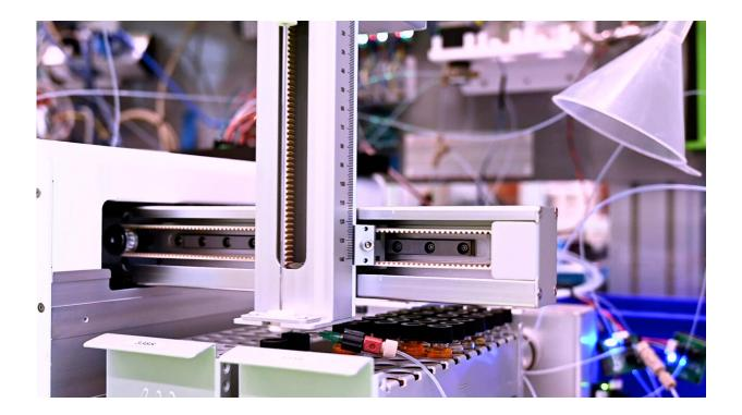
A robotic needle sampler selects precise quantities of various reagents and skilfully mixes these to create a reaction solution. Credit: University of Amsterdam
