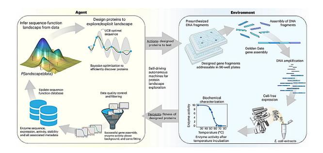
SAMPLE consists of an intelligent agent that learns sequence–function relationships and designs proteins to test hypotheses. The agent sends designed proteins to a laboratory environment that performs fully automated gene assembly, protein expression and biochemical characterization, and sends the resulting data back to the agent, which refines its understanding of the system and repeats the process. Credit: *Nature Chemical Engineering* (2024). DOI: 10.1038/s44286-023-00002-4
