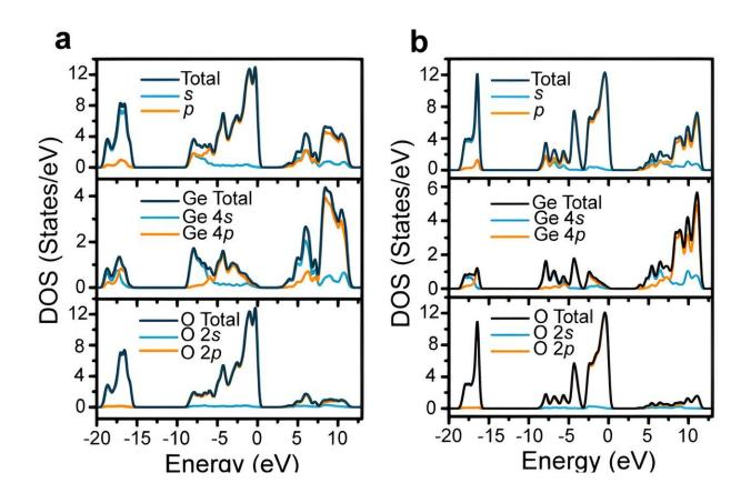
Electronic structures of the  $[GeOØ_2]n$  chain and the  $[GeØ_4]n$  network (two building units of the GeO<sub>2</sub> melt). Credit: Zheng Guimei, adapted from *Nature Communications* (2023). DOI: 10.1038/s41467-023-42890-3
