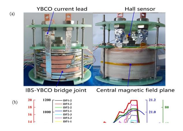
(a) The iron-based superconducting high field insert coil (b) The coil charge experiment results in 20 T background magnetic field. Credit: Ding Hangwei
