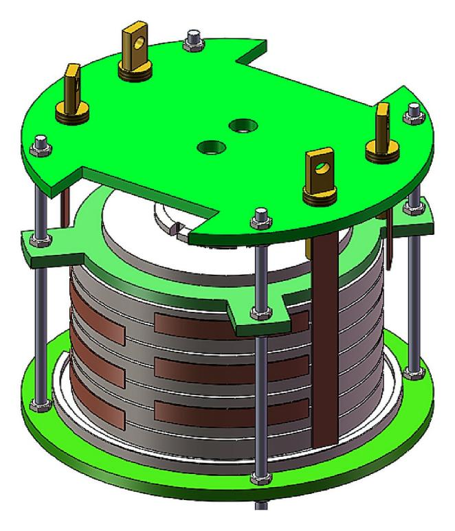
The First Tesla Class Iron-based Superconducting Coil Performed Well in High Field. Credit: Ding Hangwei
