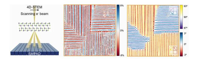
Rice researchers used four-dimensional scanning transmission electron microscopy to analyze the structure of the material (first panel from left); their analysis yielded a ferroelastic strain map of a flake of the material (second and third panels). Insets on the third panel represent polarization directions in different stripe domains. Credit: Han lab/Rice University
