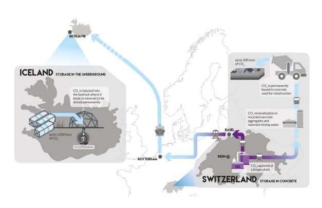
The diagram shows the process chain from  $CO_2$  capture in Switzerland to underground storage in Iceland or in concrete for construction. Credit: DemoUpCARMA / ETH Zurich
