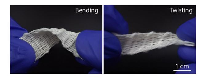
Photograph showing bending and twisting of encapsulated aerogel textile. Credit: *Science* (2023). DOI: 10.1126/science.adj8013
