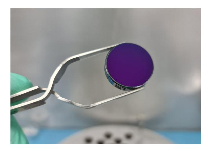
The 25mm diameter silicon substrate used for the supermirrors. The conventional base coat that has already been applied creates a purple color impression. Credit: Valentin Wittwer
