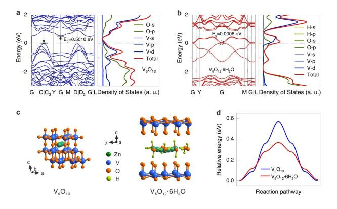
Comparison of band structure, energy gap, the density of states and diffusion energy barrier in  $V_6O_{13}$  and  $V_5O_{12}$ .<sup>6</sup>H<sub>2</sub>O. Credit: MO Li'e
