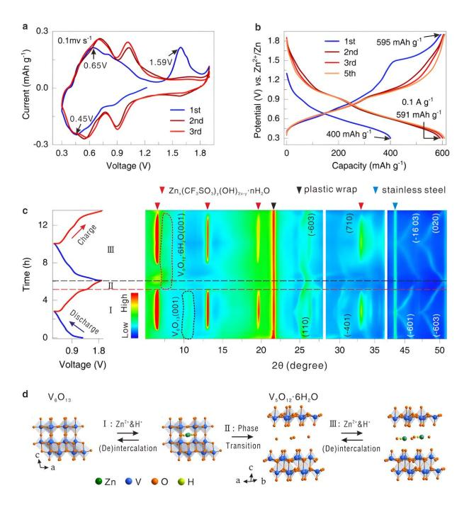
The electrochemically induced phase transformation behaviors of the  $V_6O_{13}$  cathode. Credit: Mo Li'e
