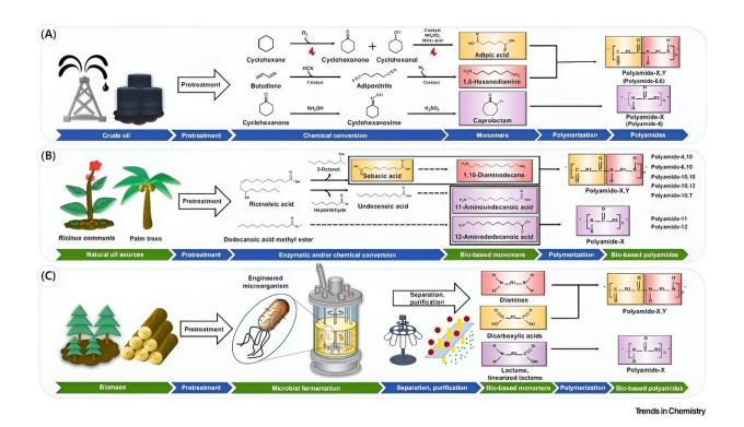
A schematic overview of the overall process for polyamides production. Credit: *Trends in Chemistry* (2023). DOI: 10.1016/j.trechm.2023.10.001
