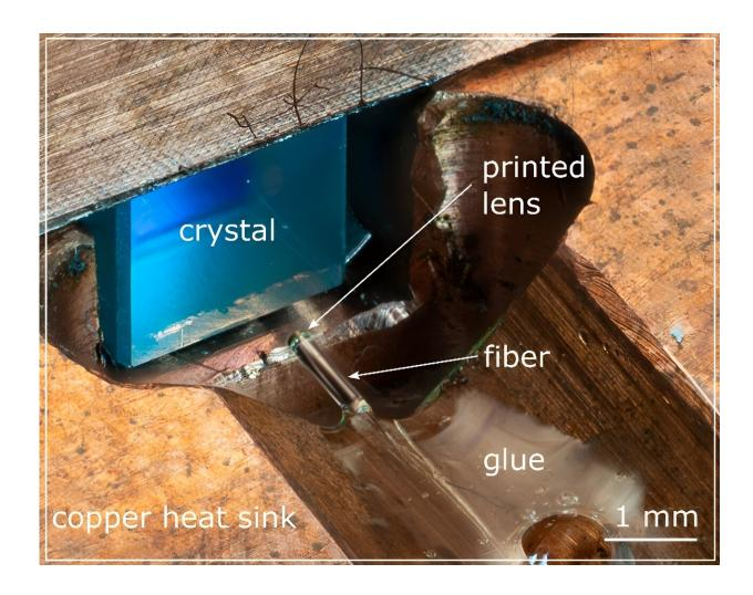
Researchers printed microscale lenses directly onto optical fibers, allowing them to compactly combine fibers and laser crystals inside a single laser oscillator. Credit: Moritz Floess and Simon Angstenberger, 4th Physics Institute at University of Stuttgart in Germany
