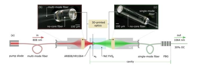
This schematic shows the laser design that uses the 3D-printed lenses for fiber coupling. The new laser combines the advantages of fiber-based and crystal-based solid-state lasers. Credit: Simon Angstenberger, 4th Physics Institute at University of Stuttgart in Germany
