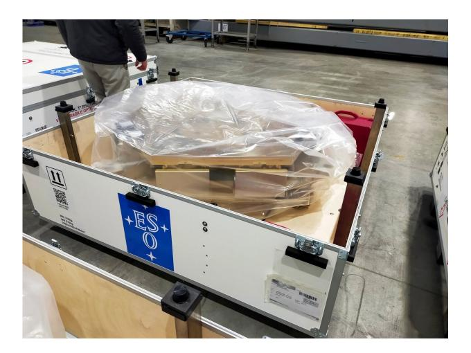
This image, taken at a storage facility near Poitiers, France, in December 2023, shows a segment of ESO's <u>Extremely Large Telescope</u> primary mirror, together with its support system, boxed and ready to start its 10 000 km long journey to Chile. Once there, the segments will be coated with a thin layer of reflective silver and stored in preparation for installation on the telescope. Each segment is close to 1.5 meters across and 5 centimeters thick, and their surfaces have been
