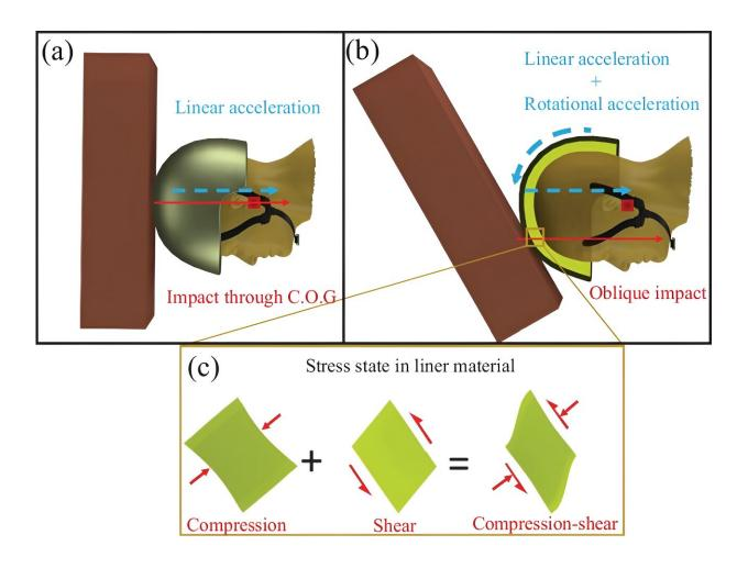
Head helmet impact kinetics and deformations induced on the protective liner: (a) An impact that acts through the center of gravity of the head-helmet system causing pure linear acceleration, (b) An impact that acts away from the center of gravity of the head-helmet system causing both linear and rotational
