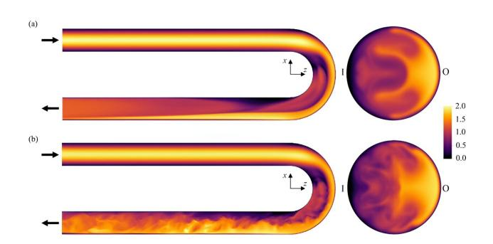
Velocity magnitude field computed via nonlinear DNS after 200 convective time units  $(D/U_b)$  at (a) Re<sub>b</sub>=2500 and (b) Re<sub>b</sub>=3000. The xz symmetry plane and the xy cross plane at z=0 (bend outlet) on the left and right, respectively. The black arrows indicate the inflow and outflow directions. The inner and outer walls are marked with letters I and O. Credit: *Physical Review Fluids* (2023). DOI: 10.1103/PhysRevFluids.8.113903
