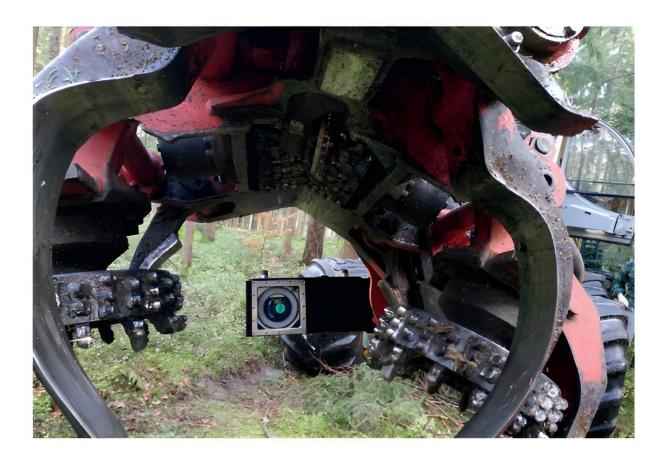
Tamper-proof traceability from the harvest to the sawmill: A camera system integrated into the forest harvester records the cut surfaces and generates a fingerprint code for each log. A second image taken later can identify the log based on a unique code. Credit: Fraunhofer IPM
