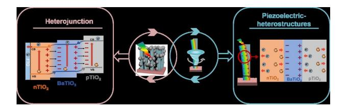
The formed built-in electric field and polarized-induced electric field at the interface of heterojunction to promote carrier separation. Credit: M. Ai et al
