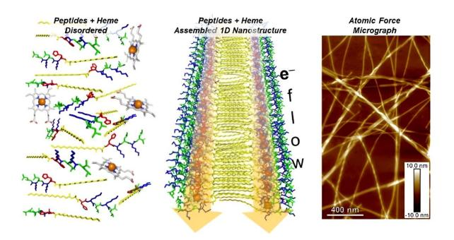
Peptide molecules and heme disordered in solution (left) are transformed into an ordered one-dimensional (1D) self-assembled nanostructure (center) that supports electron flow, as imaged by Atomic Force Microscopy (right). Credit: Argonne National Laboratory
