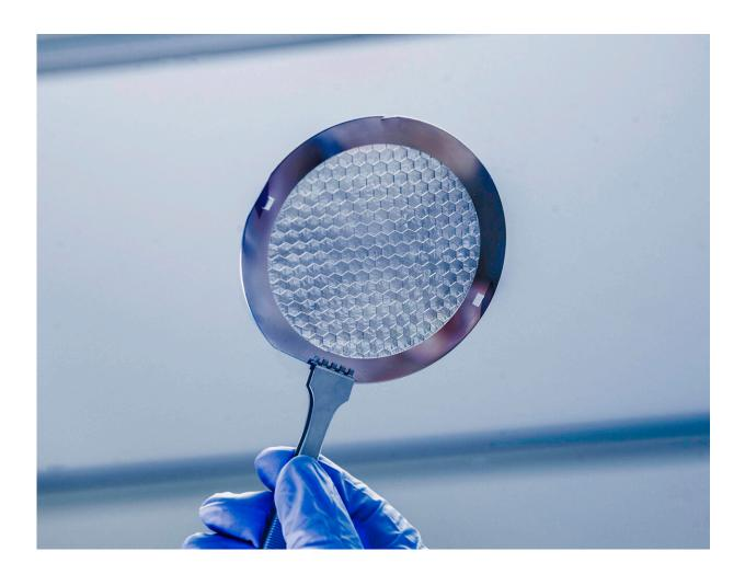
Photon sieves like this are cut from a single wafer of silicon or niobium to focus extreme ultraviolet light—a difficult wavelength to capture. Credit: NASA / Christopher Gunn
