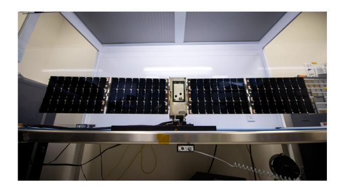
The BurstCube satellite sits in its flight configuration in this photo. The shoebox-size spacecraft will launch aboard a resupply mission to the International Space Station, where it will be released into orbit. The solar panels on either side will deploy after it leaves the station. Credit: NASA/Sophia Roberts
