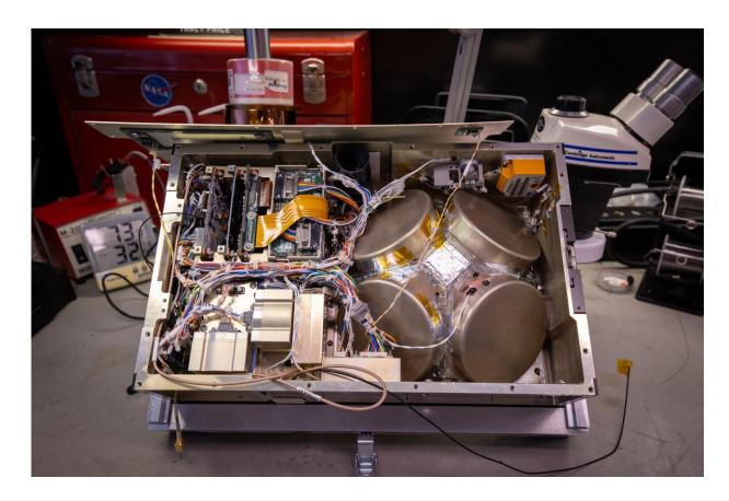
Interior components of the BurstCube satellite appear in this photograph. BurstCube, a shoebox-sized satellite that will study some of the universe's most powerful explosions, was designed and built at NASA's Goddard Space Flight Center in Greenbelt, Maryland. The four circular detectors make up the mission's gamma-ray detector. Credit: NASA/Jeanette Kazmierczak
