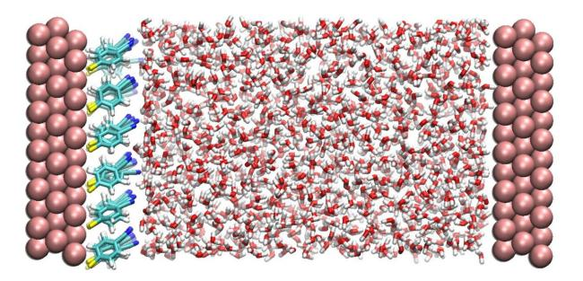
A snapshot taken from the computer simulation model of the system in this study. On both sides are three layers of gold atoms representing the metal electrode with adsorbed organic molecules on the left electrode. The space between the electrodes is filled with water molecules. Credit: Institute for Basic Science
