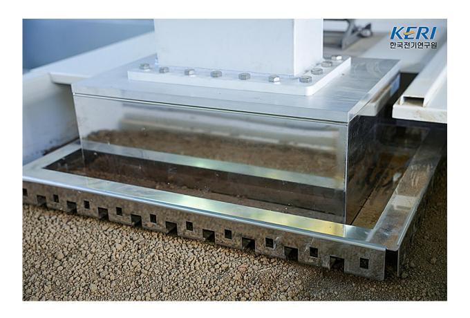
An antenna (radiatior) that heats the soil by penetrating microwaves to depths of 30 cm or more underground. Credit: Korea Electrotechnology Research Institute
