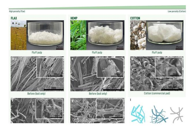
Morphology of single fibers from different fiber-rich plants effects absorption capacity. Credit: *Communications Engineering* (2023). DOI: 10.1038/s44172-023-00130-y
